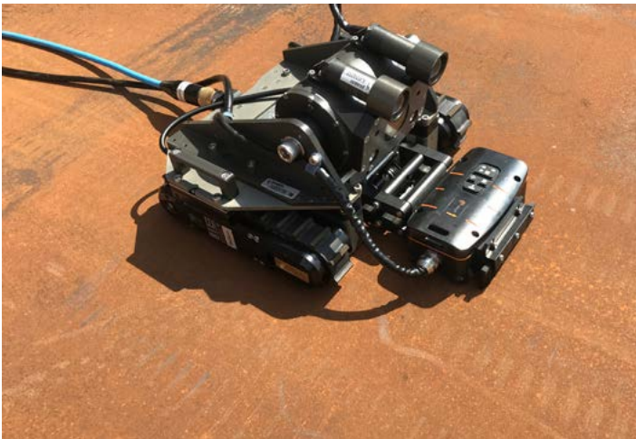
Customized Magg crawler with Eddyfi Sharck ECA Probe
