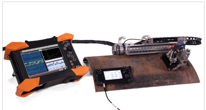
Figure 9 and 10: Automated crawler for corrosion and weld inspection. Handles removable.
