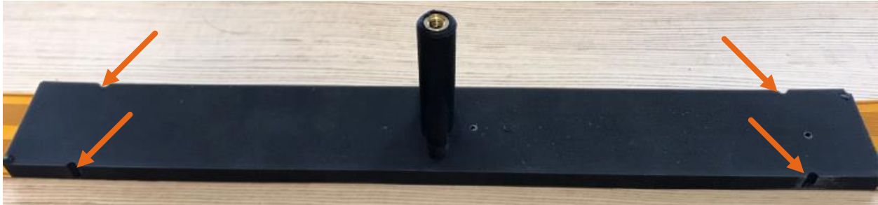
Figure 4. Four indicators of coverage on the Spynet probes.
