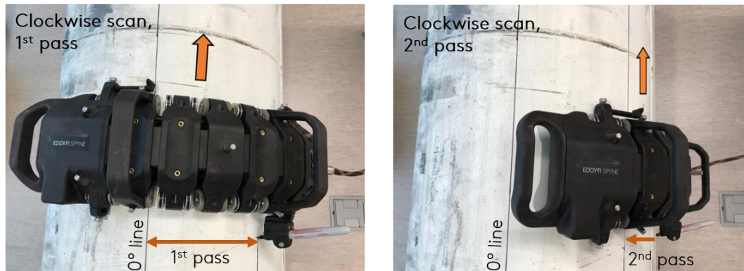
Figure 15. Clockwise scans with the pointer on the left side. The pointer at the front of the Spine follows the 0° line during the first pass and follows the next bottom line during the subsequent passes.
