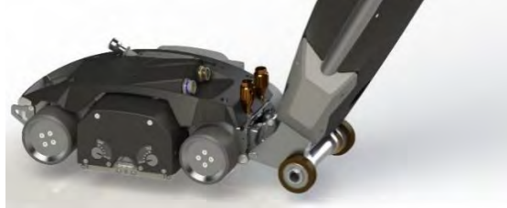
Figure 21: Engaging the mainframe with the scanning head
