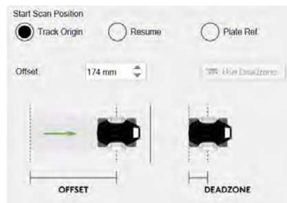
Figure 80: Start scan position - track origin
