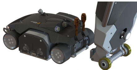
Figure 20: Offering the mainframe to the scanning head
