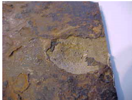
Left to right: Underside of floor cutouts showing underfloor corrosion; characteristic circular staining around weld highlights pinhole type leak
