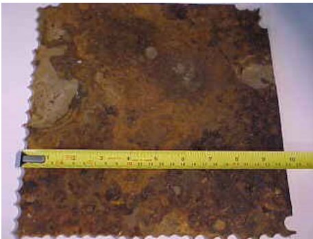
Left to right: Underside of floor cutouts showing underfloor corrosion; characteristic circular staining around weld highlights pinhole type leak
