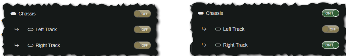
FIGURE 43: DISABLING THE WHOLE CHASSIS OR AN INDIVIDUAL TRACK
