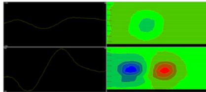
20x2 mm (0.79x0.08 in) defect in carbon steel detected through 12 mm (0.47 in) neoprene coating
