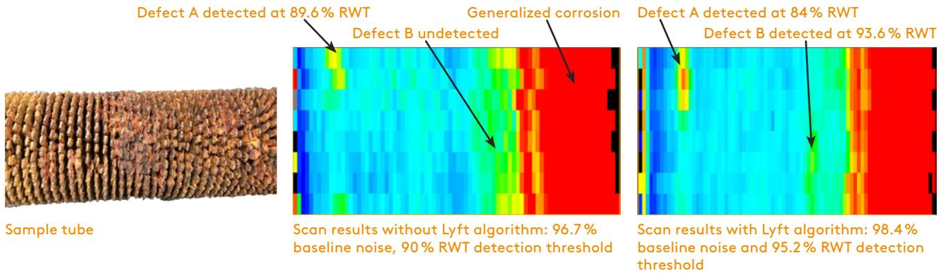
the volume of the probe's estimated smallest detectable defect. It was positioned at 12 o'clock, 152.4mm (6in) from the cut out end of the tube. It was about 0.84mm (0.033in) deep with an area of 645.2mm<sup>2</sup> (1in<sup>2</sup>).
