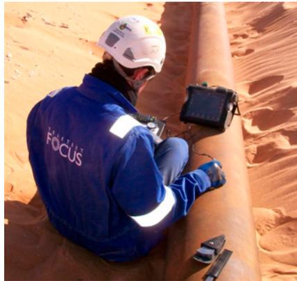
**Ultrasonic wall thickness scans performed at FOCUS+ tool locations and at corroded areas to confirm internal corrosion was not present**
