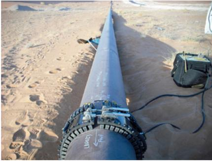
**FOCUS+ guided wave ultrasonic test equipment used to inspect an 45.7 cm (18 in) trunkline of the MLN field in Algeria**
