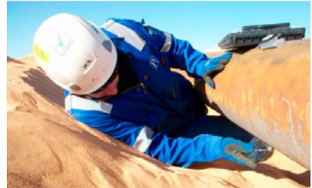
**Characterizing external pitting corrosion using pipe pit depth gauges (lever type and dial gauge)**
