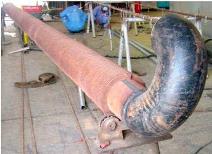
A defect was ground into the center of the pipe and FOCUS+ was used to see whether this could be detected.
