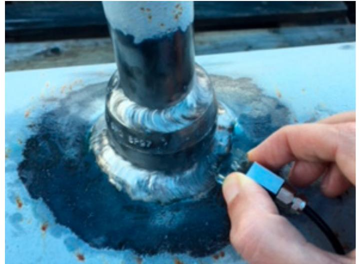
Manual scanning of nozzle welds is challenging
