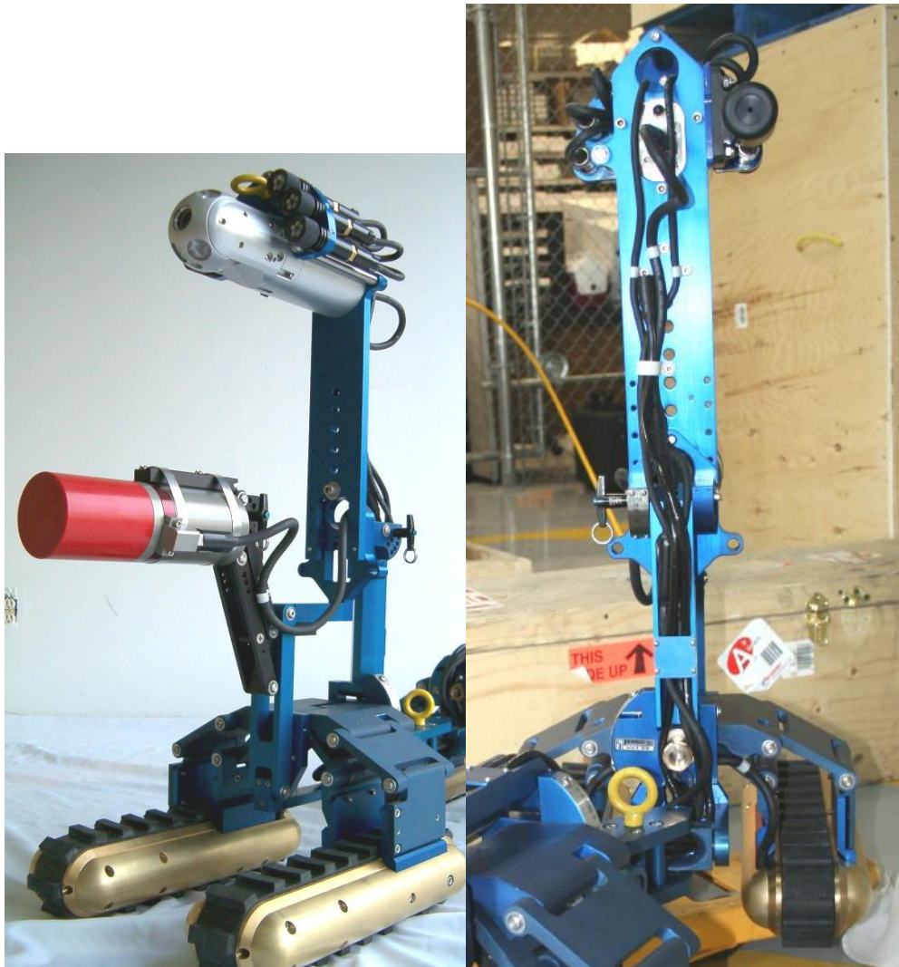
FIGURE 26: EXTENSION BRACKET WIRE ROUTING
