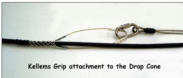
FIGURE 6: KELLEM'S GRIP/TOW CABLE ASSEMBLY
