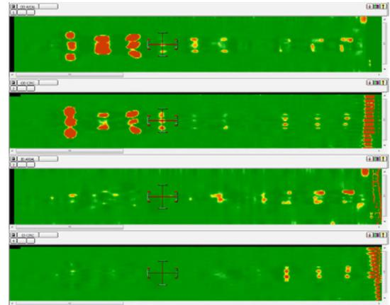
simple to locate defects along a weld's length.
