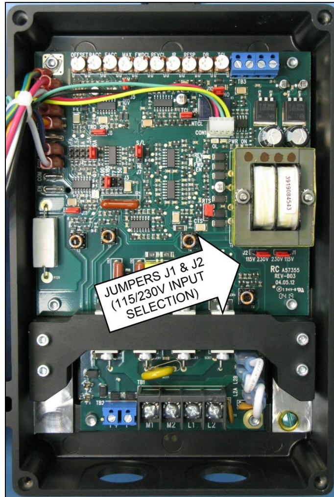
FIGURE 5: LINE VOLTAGE SELECTION, JUMPERS J1 AND J2
