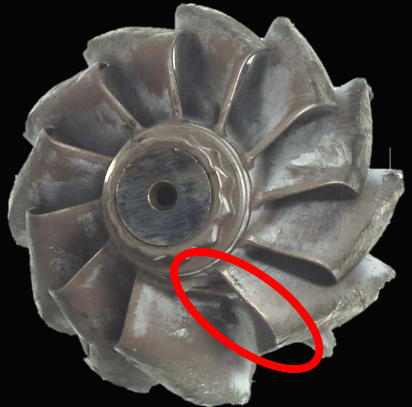
Failed Turbine Wheel
